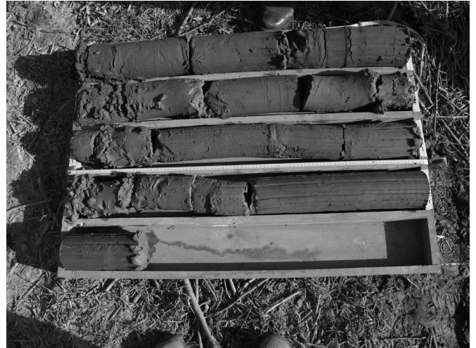
Fig. 3 Extruded boring cores, 1 metre in length and 127 mm in diameter, were placed into the wooden container.
